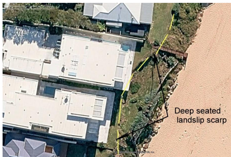
P3.3: Deep seated landslip; 93 to 97 Ocean View Drive
