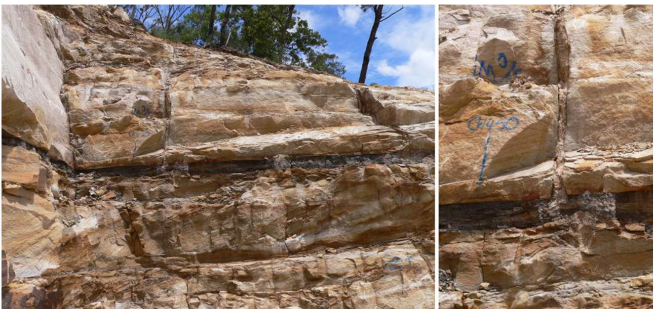
Fig. 2. Photographs of the abutment of Shannon Creek Dam, showing in-filled stress relief joints. The joints are up to 80 mm wide and terminate on shale beds. Photographs courtesy of L. McDonald and Clarence Valley Council (Fell et al. 2015).
