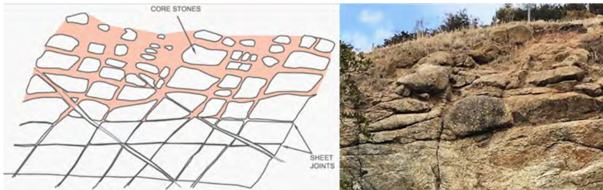
Figure 12: Conceptual engineering geology model for a granitic rock mass
