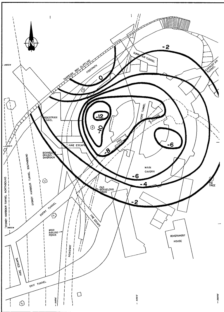
Figure 5. Contours of surface settlement.
