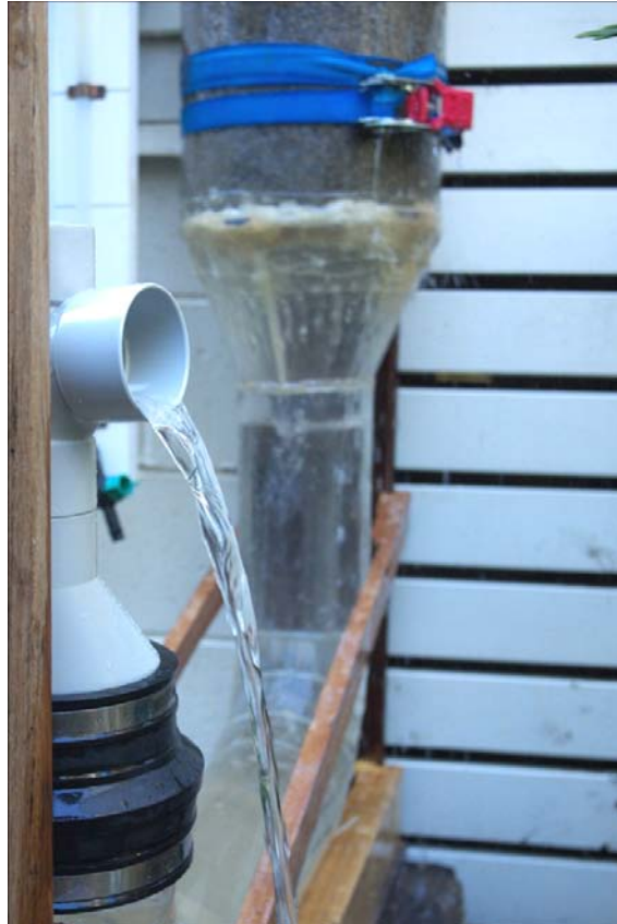
Figure 13: Final test; water allowed to cascade from base of column
